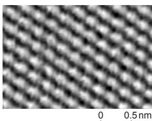
This tunnelling effect has also led to microscopes that can "see" individual atoms e.g. the graphite atoms in the hexagonal pattern in the image.
